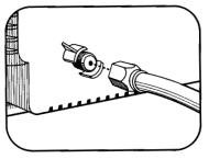
If your cable system does not require the use of a cable box, simply press or screw the incoming cable onto the antenna terminal on the back your TV. If your cable system requires you to use a converter box for all channels, connect the incoming cable to the IN terminal on the converter box. Connect another cable between the OUT terminal on the converter box and the antenna terminal on the TV. You will need to keep your TV tuned to channel 3 or 4 and change channels using the converter box.
